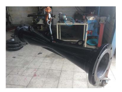
**WEIZEN** is designed and manufactured the venturi tube in full compliance with ISO 5167 and ASME MFC-3M standards.
